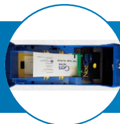
Enclosure opens directly to the paper path
